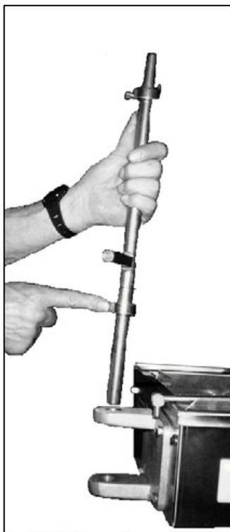
Figure 1-3. Inserting the Swing Column.
