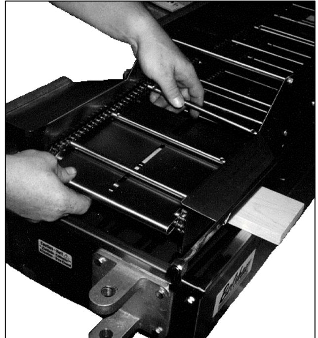
Figure 3-4. Removing the Drop Plate.
