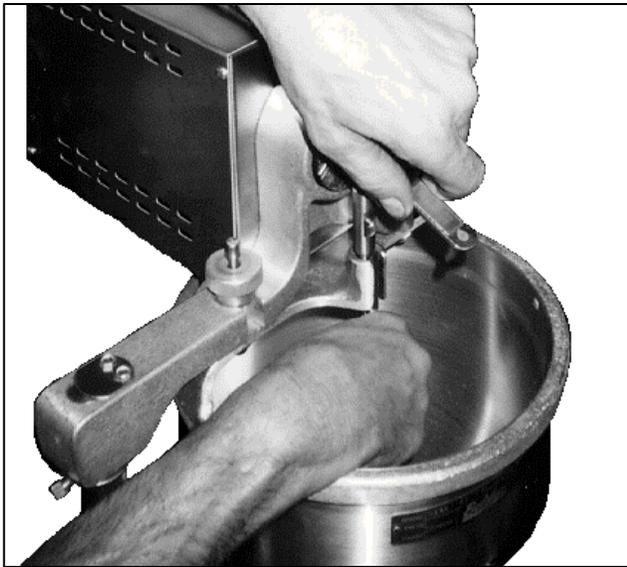
Figure 1-7. Installing the Plunger.
