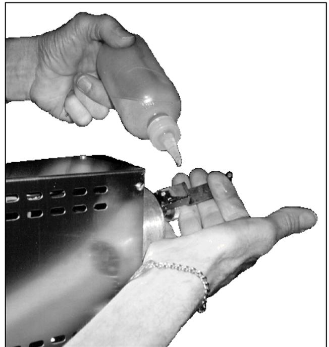
Figure 4-1. Lubricating the Connecting Rod.
