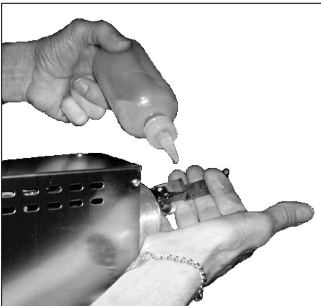
Figure 2-1. Lubricating the Connecting Rod.
