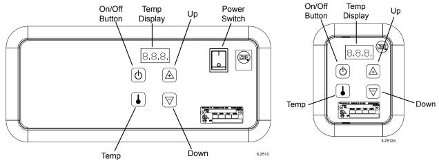
Left: Typical Electronic Autofill Controls Unit Right: Typical Electonic Controls Unit
