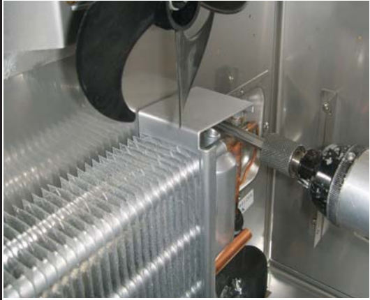
A.Remove the evaporator coil
