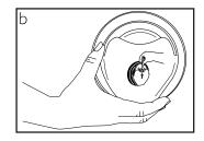
I. Open lid dispenser door by pressing down on top of door assembly (a) and pulling outward (b), releasing door latch.
