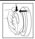
2. Load full sleeve of lids, assuring that inside of lids are facing outward, as shown.
