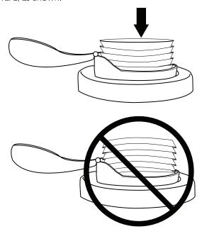
3. While holding lids in place, close lid dispenser door, snapping latch securely in place.
