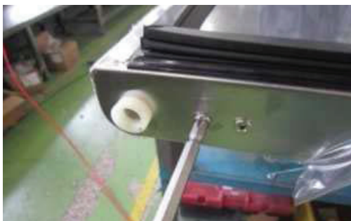
F. Disassemble stopper plate, then tight screws.
