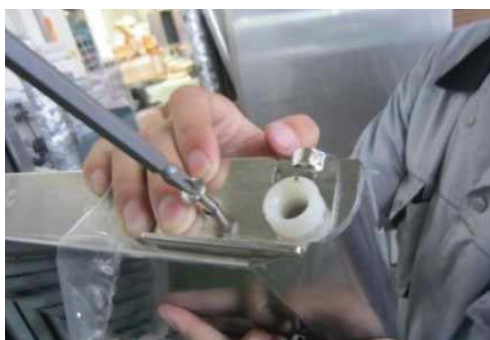
G. Assemble stopper plate in original positions.
