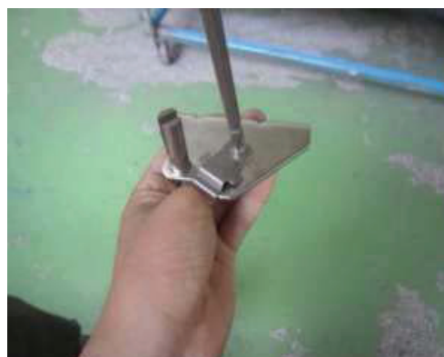
D. Screw stopper plate on top hinge (right).
