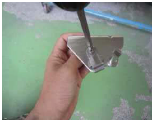
C-2. Disassemble bottom hinge (left).
