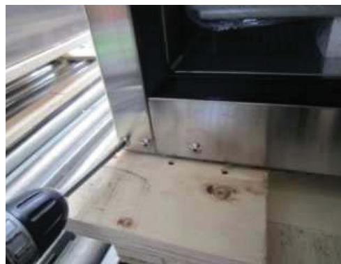
C-2. Disassemble bottom hinge (left).
