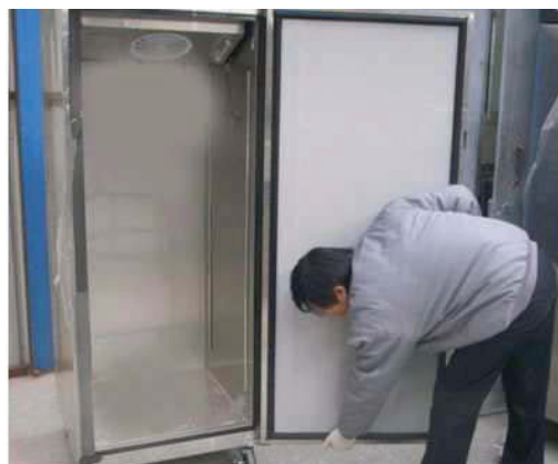
B. Lift the door, then remove it.
